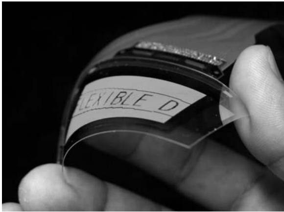
Figure 9.30 A photograph of a passive matrix OLED display on a polymer substrate.
