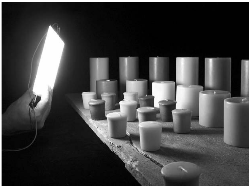
Figure 10.9 A white light OLED research device made at GE Global Research, which provides 70 lm of illumination with a color temperature of 4000 K, a color rendition index of 90, and an efficiency of 7 lm/W.
